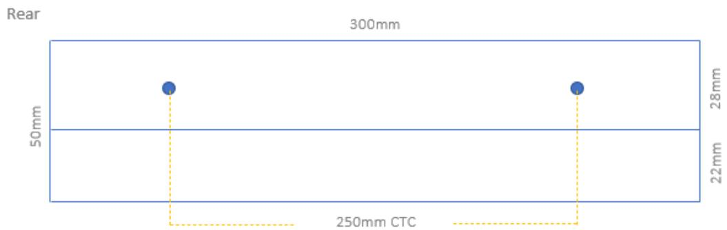
b) Locate and mark the top position for the handles on the door.
