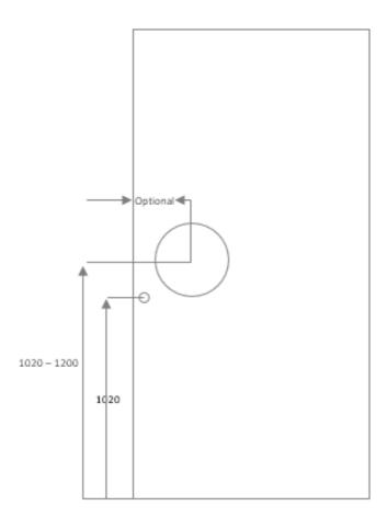
b) Referring to the chart below, drill a hole through the door at the point marked out above
