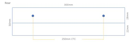
c) Drill \*two holes <u>in the door</u> to suit the <u>diameter and depth</u> of the dowel supplied. E.g. for a 12mm dowel, drill a 13mm hole.
