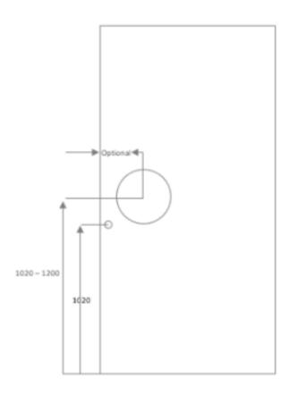
b) Referring to the chart below, drill a hole through the door at the point marked out above \*Be sure to check the size of the fitting prior to drilling.
