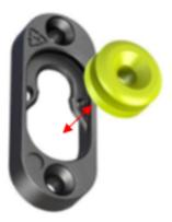
d) With the handle flush against the door face, slide it downward until it 'clicks' past the neck and locks into the smaller section of the keyhole fitting.
